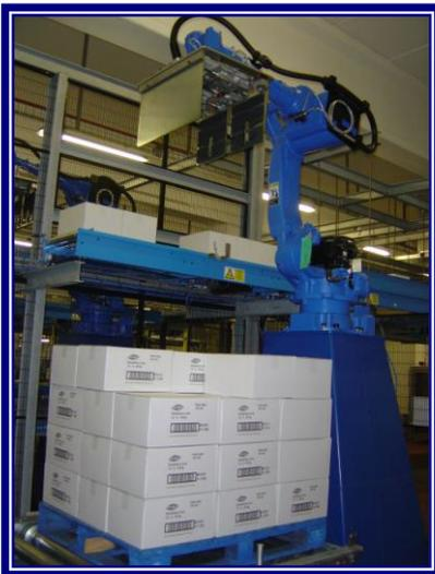
The ground floor houses all case packing and palletising operations. Compere supply starts post packer and comprises 4 spiral elevators, slat and roller conveyors, 4 articulating arm robots, empty and full pallet distribution, stretch wrapping and labelling.
